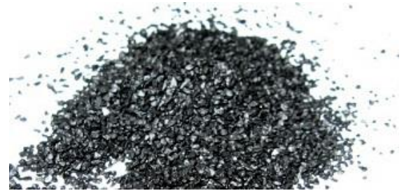
Black Powder: S, C, KNO 3 probably invented by Chinese alchemists searching for Elixir of Life
